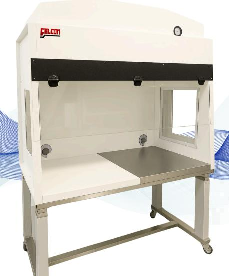
Our FELLAB Bench-Mounted Vertical Laminar Flow Cabinet features a twostage filtration system for maximum cleanliness and protection. The first stage provides efficient pre-filtration, while the second stage uses an absolute HEPA filter to deliver particle-free airflow. Each unit includes a manual fan speed controller to adjust for filter loading and a filter condition indicator for easy maintenance. Often held in stock.
