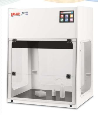
been designed as an ideal environment for the manipulation of DNA and RNA, especially for the setup of PCR assays. An integrated UV lamp enables rapid decontamination of the work zone between experiments and prevents cross-contamination. HEPA filtered clean air across the entire worksurface ensures an ultraclean operational environment.
